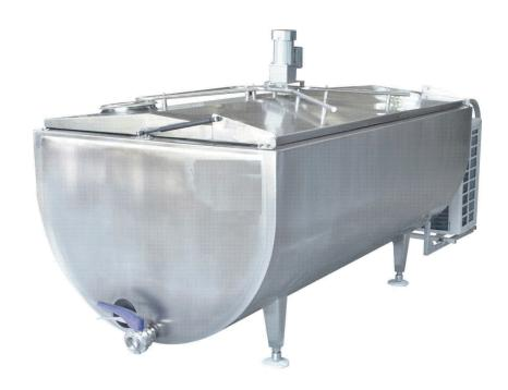
Milk Cooling Tank Bulk Cooler 1000 Ltrs Direct Expansion Cooling Tank (Open Tank Semi Cylindrical Rectangular Shape) capacity 1000 Liters has large opening lids for easy access and rounded internal corners, to facilitate thorough cleaning. Tank insulation is provided by factory injected polyurethane foam of 50 mm. The integral condensing unit is Hermetic Type with R22 refrigerant. Condensing unit Stand is made of Galvanized Anti Rust Steel. It occupies little space.
